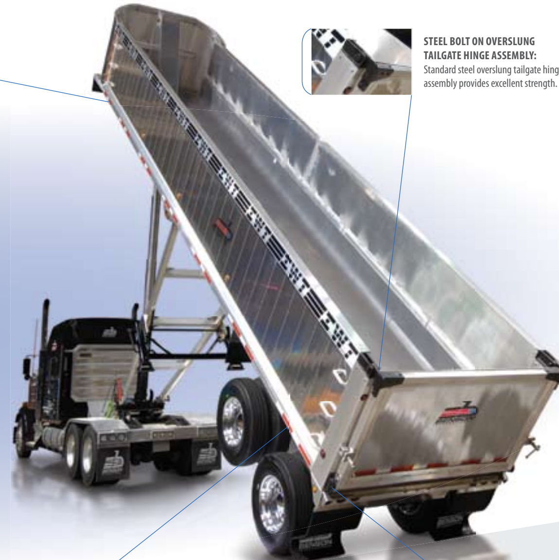
EXTRUDED ALUMINUM SUB FRAME: 17" Deep Aluminum Extruded Sub Frame.
